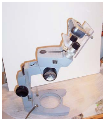
Figure 2: Adapter, digital camera, and microscope.
