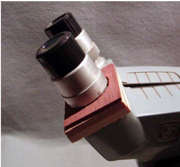
Figure 5: Basswood adapter “stop” on microscope
