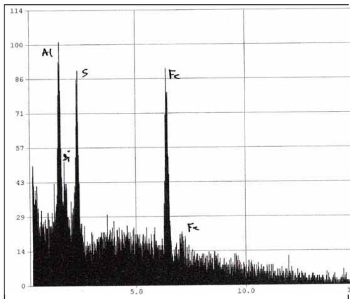
The EDS spectrum, to the left, for the white, crusty mineral indicated an Iron Aluminum Sulfur species.
